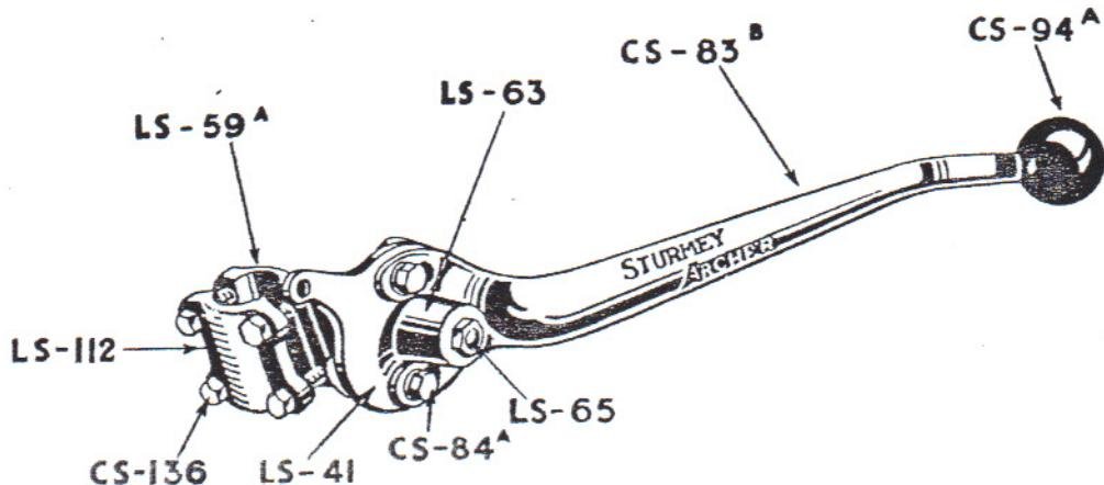
This type of control can be supplied to fix to the Saddle-down tube as illustrated above, or mounted on a bracket bolted to the top of the box, or fitted to an extension of the gearbox cover.
